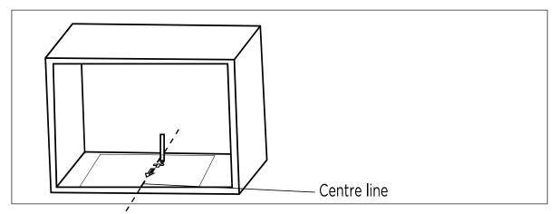
• Remove the bottom cabinet template and fix the mounting plate with screw.
